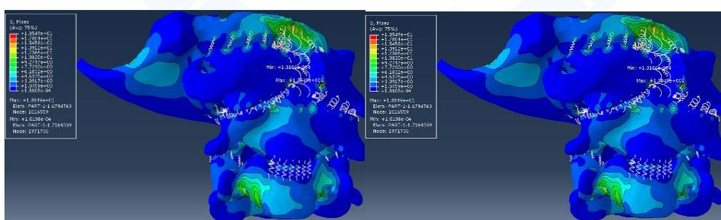
Fig. 4 Comparison of stress distribution between intact and fractured transverse ligaments in composite fractures of the atlas axis
